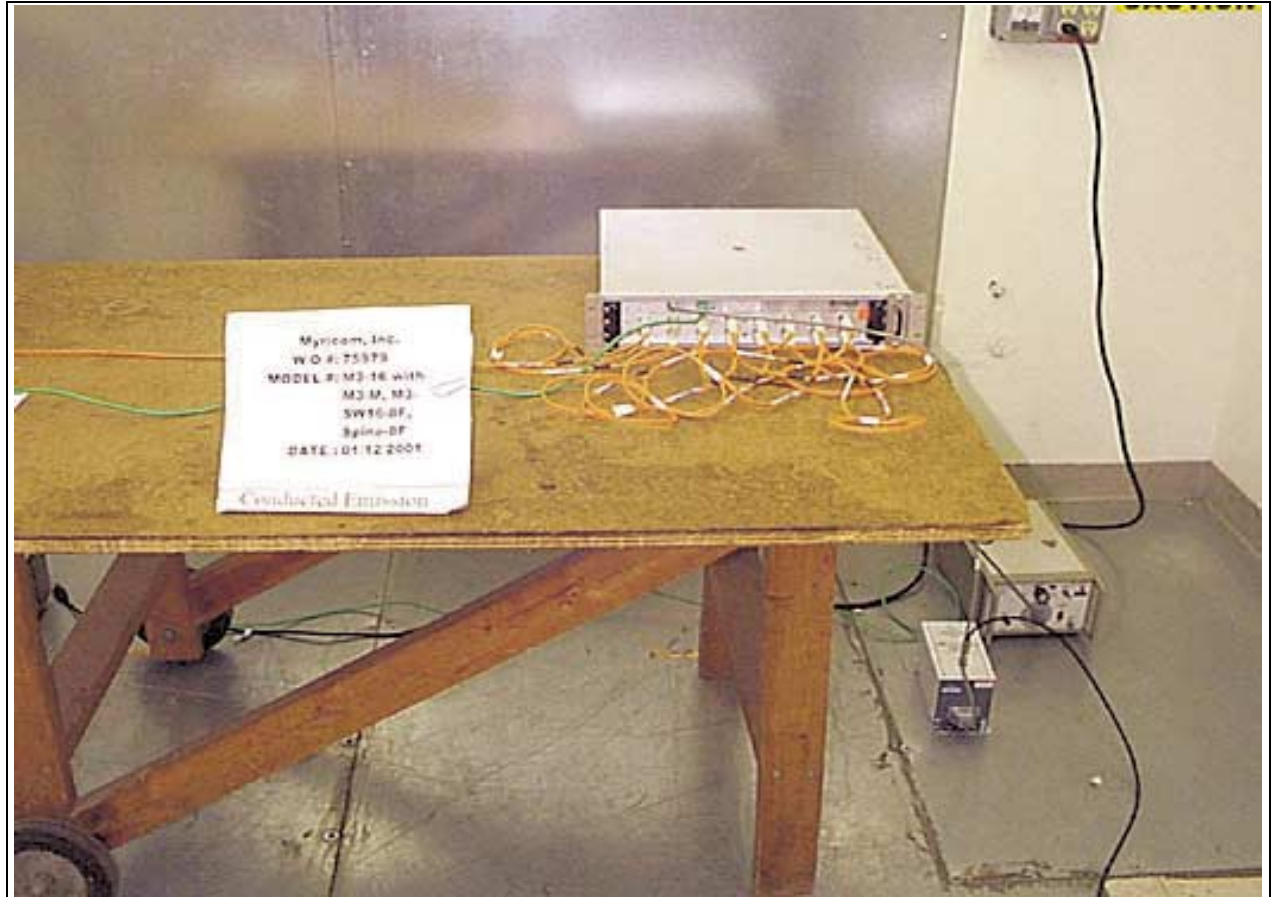
Conducted Emissions - Front View (Telecom)
